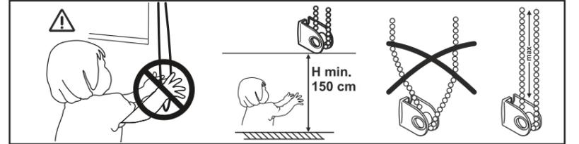
**EN** Read these instructions carefully before installing and using the safety device. Children can be strangled if the device is not installed correctly. This safety device shall be correctly installed for the protection from strangulation of young children and the proper operation of the blind. Keep the instructions for future reference. Use of safety devices helps reduce the risk of strangulation but cannot be considered entirely foolproof.
